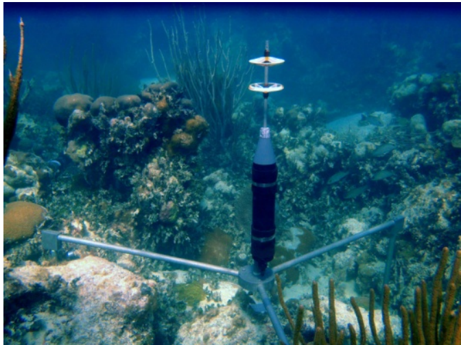
CROSS (Coral Reef Oxygen Sensing System) at Cheeca Rocks, Florida Reef Tract Class III NCRMP/OAP monitoring site
