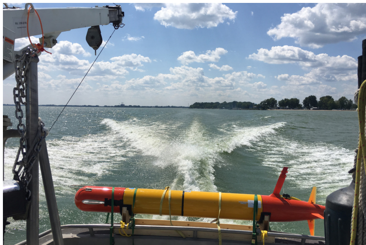
Scientists deploy underwater autonomous vehicles to test environmental sampling for 'Omics research in Lake Erie. Photo Credit: NOAA, GLERL.
