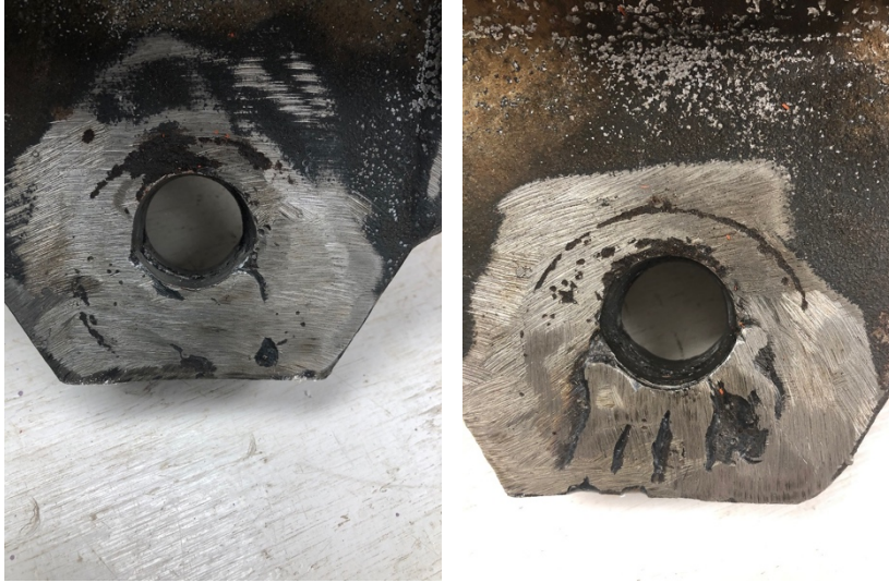
Figure 2 Refurbished (left) and old (right) bridle yoke.
