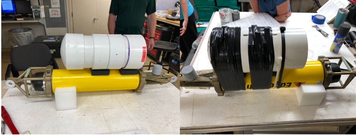
Figure 5 Sargassum container (white) attached to the acoustic release (yellow) before (left) and after (right) securing with tie wraps and electrical tape.
