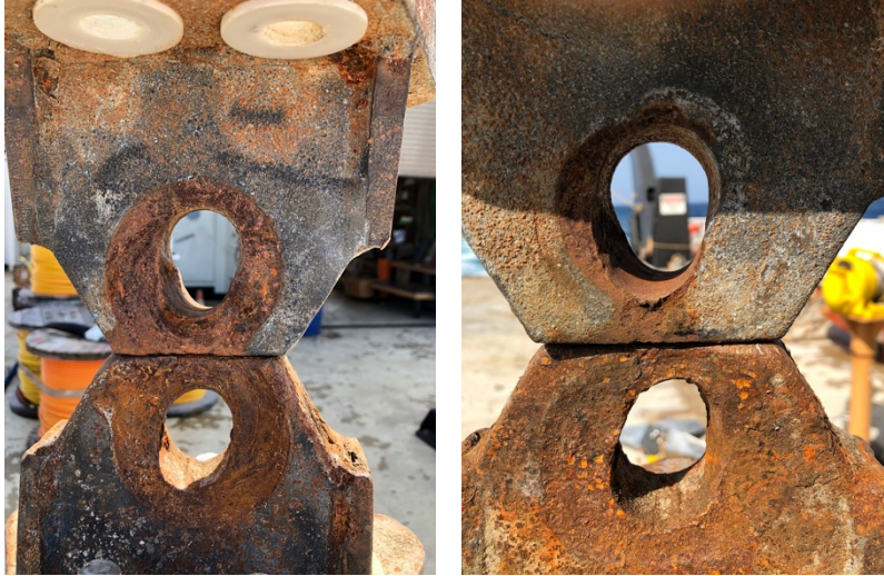
Figure 3 Wear on mooring bridle yokes.
