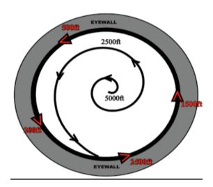
Primary Objective: Sample the highest winds of the TC at various altitudes within the eyewall.
