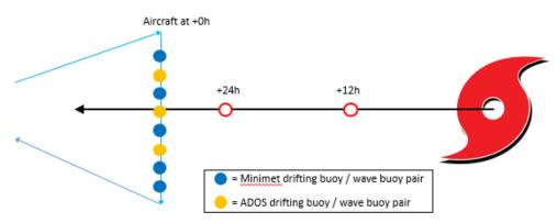
*Figure 3. A-sized DWSB drifters*. *Representative deployment line of drifter pairs 24h ahead of the arrival of gale-force winds, from a C-130J.*
