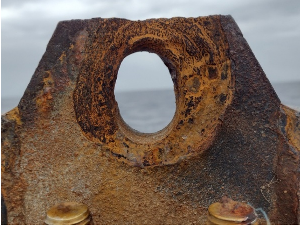
Figure 6. Worn clevis from 12°N, 38°W (PI254) recovery.
